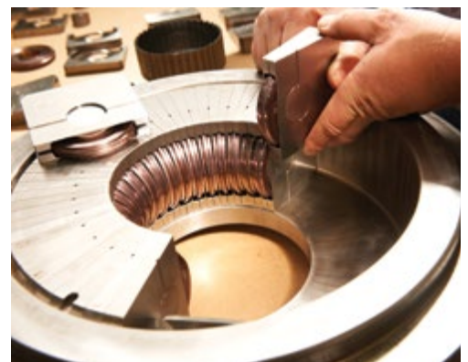
Roller die – at the core of the technology are forming rolls – arranged in pie-shaped cassettes encapsulating a part 360 degrees.
