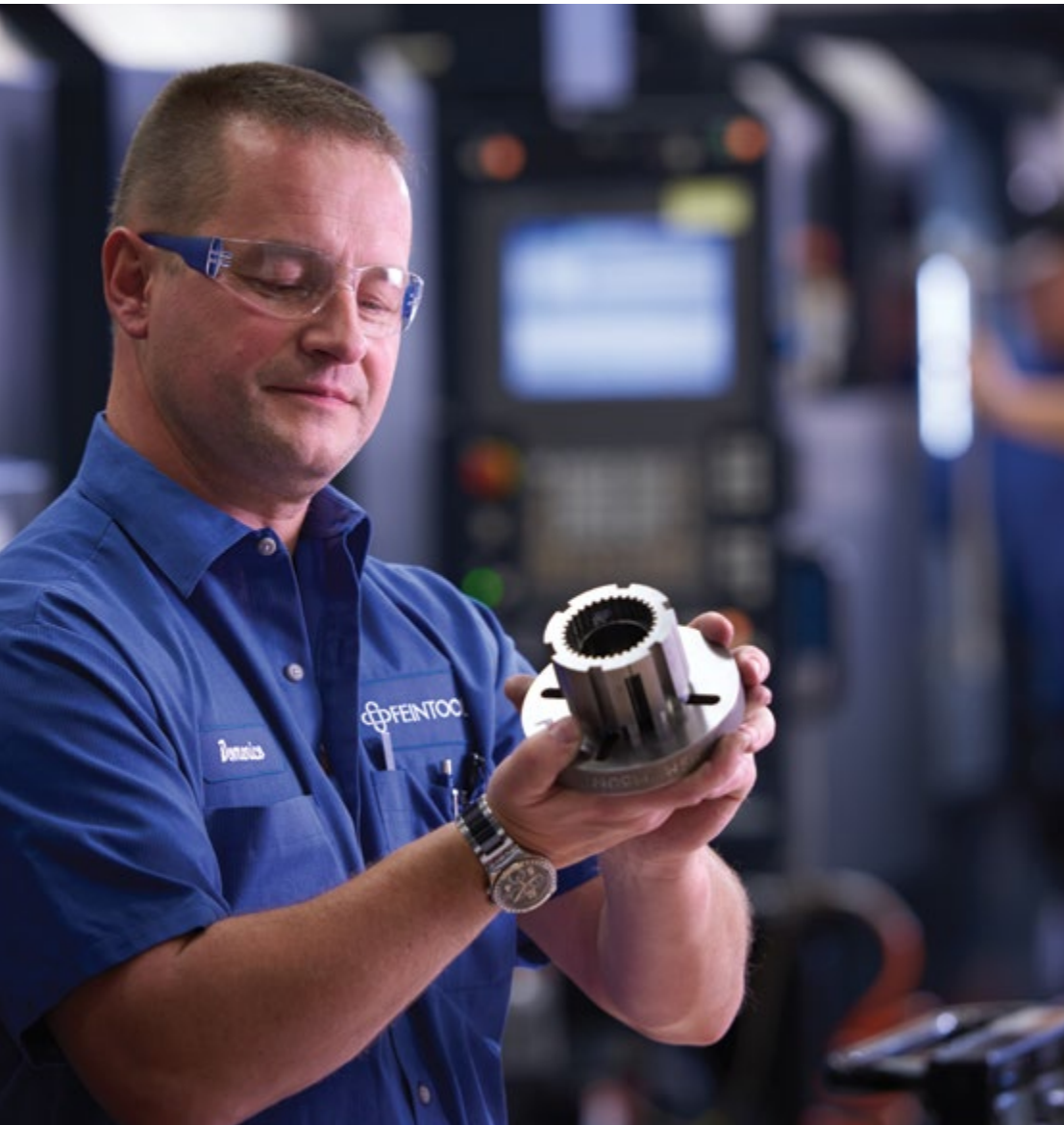
The dies used in fineblanking are modular, with the individual components assembled after hard milling. This enables Feintool to replace or refinish individual components rather than the entire die as it sees use over time.
