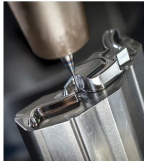
Moving to hard milling essentially eliminated all hand work for Feintool's die components. This drastically improved the repeatability of the process when it came to reworking or replacing die components.
