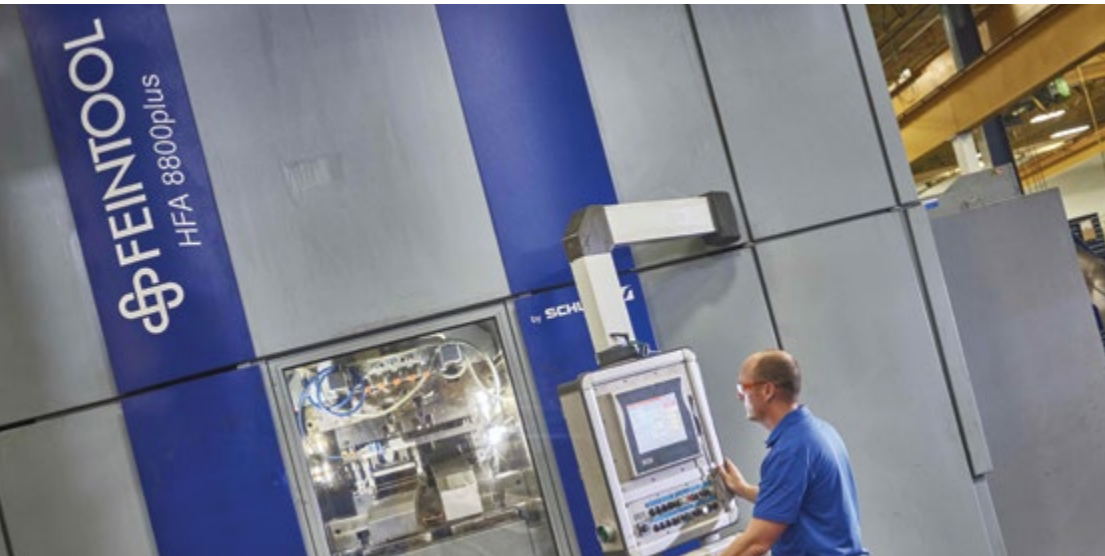
Latest generation 8800-ton fineblanking press running two-out clutch plates with up to 60 strokes per minute.
