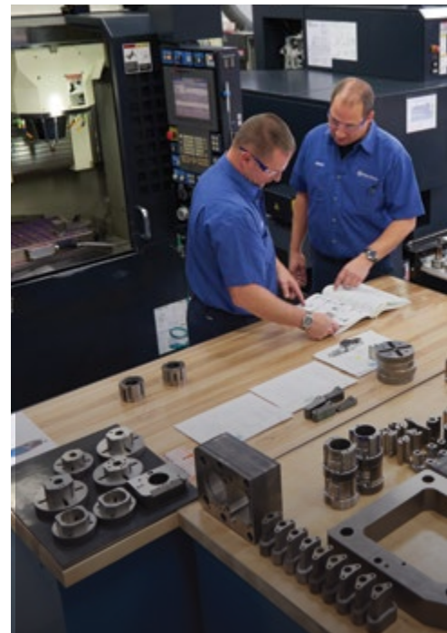
Moving to hard milling essentially eliminated all hand work for Feintool's die components. This drastically improved the repeatability of the process when it came to reworking or replacing die components.
