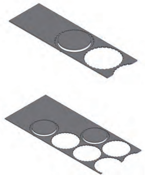
Improved strip layout delivers 7.9% material saving. (Part example: O.D. 145mm, thickness 4.2mm, 1-out usage 1.723 lbs./part, 2-out usage 1.587 lbs./part)
