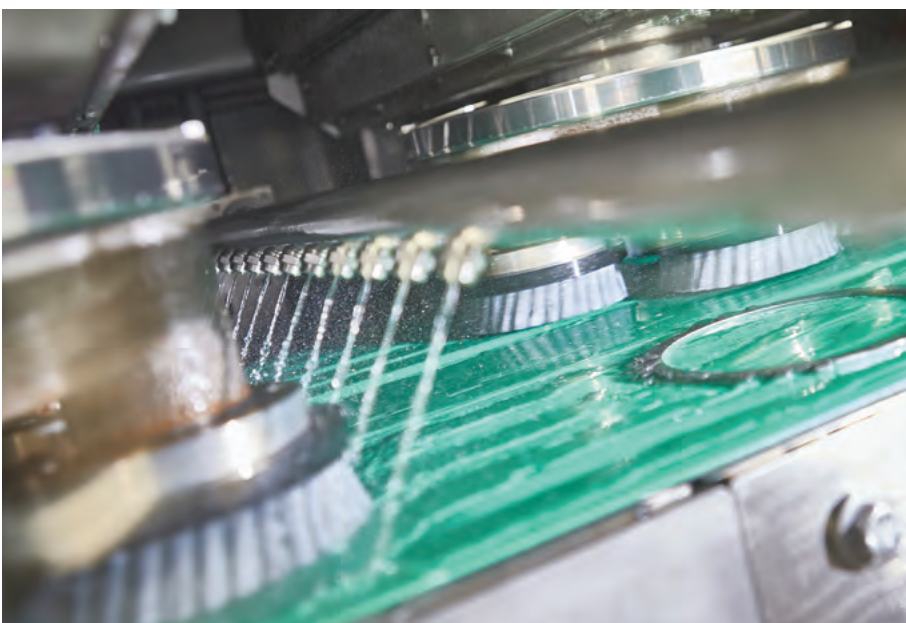
Automated planetary brush deburring/brush surface preparation process
