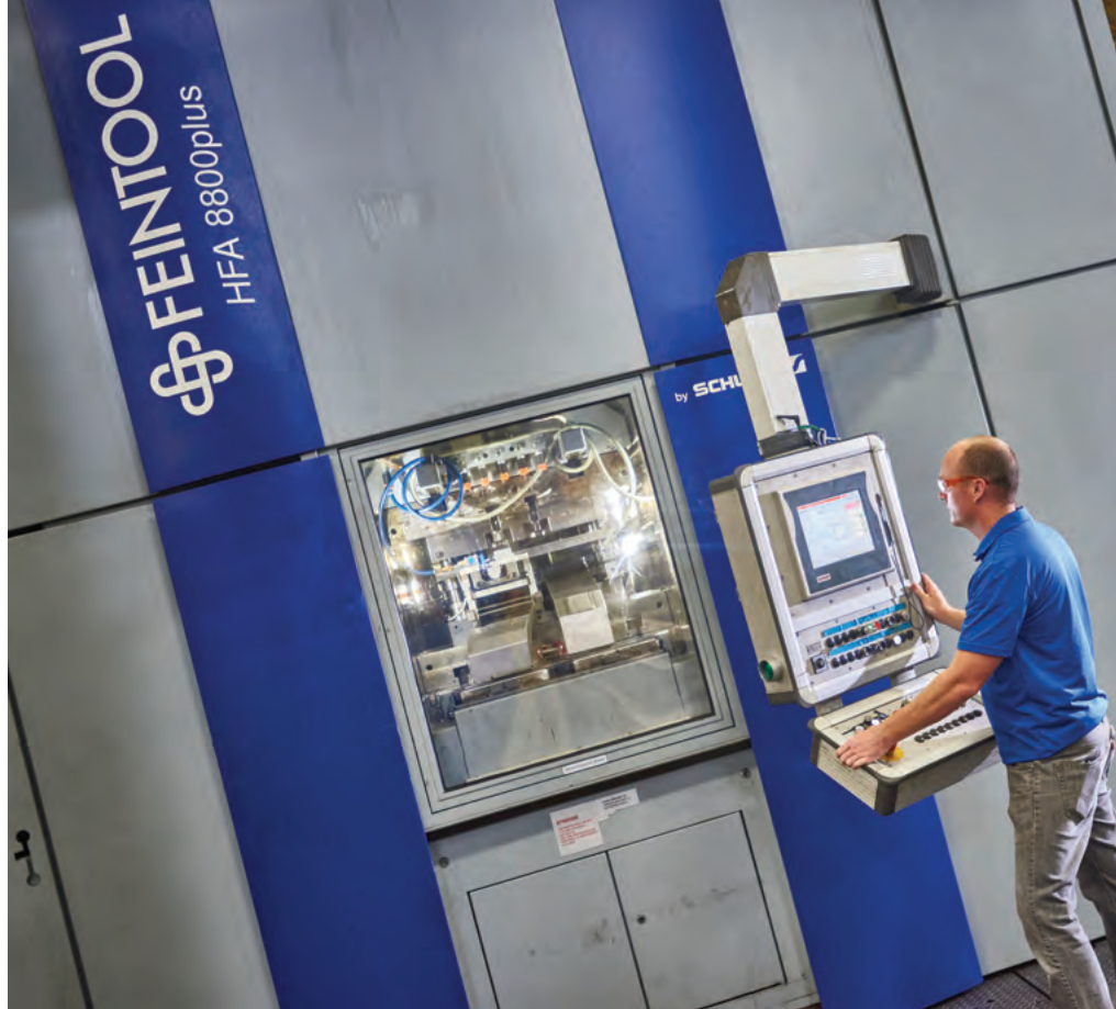
FeinClutch fineblanking tool installed in an 880-ton Feintool fineblanking line
